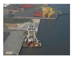
Conventional transport by installation ships or pontoons is not the only way to ship foundation piles to the offshore site. Since mid-August, Cuxport supports the Dutch installation company Ballast Nedam Offshore for the E.on project 'Amrumbank West' with an alternative transport technology. The monopiles are lowered into the water in Cuxhaven by a shore crane and towed by a tug to the offshore construction site. On arrival at the offshore site 'Amrumbank West',
